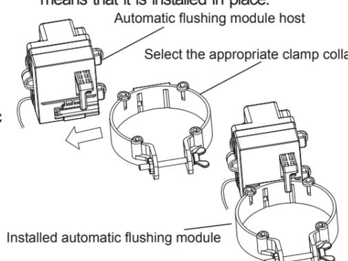
Automatic flushing module host
