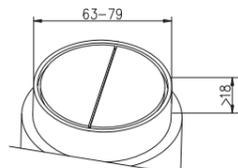
4. Select the clamp according to the measured outer diameter of the top of the fitting. When the outer diameter of the top of the fitting is from 63 to 72, select the small clamp collar. When the outer diameter of the top of the fitting is from 73 to 79, select the large clamp collar.
